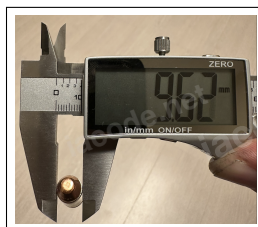
Figure 9: Caliper measurement for case mouth diameter verification.
