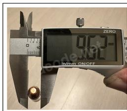
Figure 9: Caliper measurement for case mouth diameter verification.
