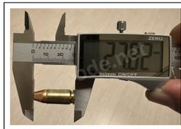
Figure 8: Caliper measurement for OAL verification.
